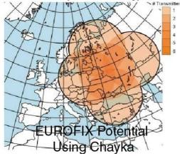
speed data reliable over ranges up to 1,500 km. The normal navigation operational mode of Loran-C and Chayka respectively is preserved which gives the Eurofix user, next to accurate DGPS positions, improved navigation reliability. As the Loran-C and Chayka infrastructure are already available, the upgrading to Eurofix is a minor and low-cost operation. Eurofix is operated by NELS. The service is free of charge for all users.
