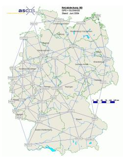
The Ruhrgas AG provides real time correction data for GPS and GLONASS positioning under the brand name ascos. Data for post processing are available as well. In close co-operation with the SAPOS reference stations the service can be provided Germany-wide. Correction data are transmitted via GSM in RTCM format at a rate of 1 second. The data are neither compressed nor encrypted.
