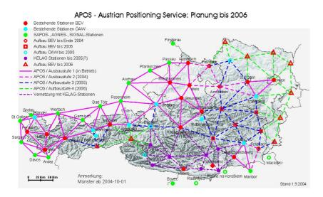
The service of APOS (Austrian Positioning Service) started in 2003 and will be made public in 2006. There are at present more than 36 reference stations and when complete there will be between 70 and 75 offering two levels of service.
