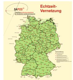
reference stations forms the basis of this system. This service is available with high reliability. SAPOS HEPS High-Precision Real Time Positioning Service offers real time positioning with accuracy of 1-5 centimetres. The user may, in addition to the EPS correction also have resource to the carrier phase correction data of the satellite signals in real time which supports precise positioning.
