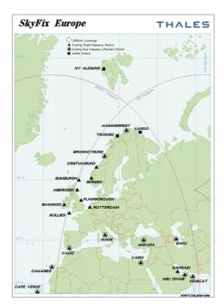
SkyFix-XP service is a more accurate DGPS service that allows users to derive positions with decimetre level precision. The service is based around corrections to the broadcast GPS orbit and clock information. This technique is therefore called Satellite Differential GPS (SDGPS) as the differential corrections are for the actual satellites, as opposed to a geographical area.
