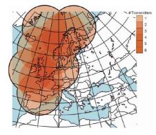
North west Europe it is run as the NELS (North West European Loran-C System) and partially available within the Mediterranean under the SELS (Southern European Loran-C System (missing stations in Spain and Turkey). Loran-C can also be used for precise time interval and highly accurate frequency applications.
